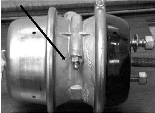
3. Insert the detachable release bolt through hole in head. Turn the release bolt clockwise until it stops and locks, then pull the release bolt out as far as possible, and run the nut down, holding the bolt in place. Using a hand wrench, turn the release bolt nut clockwise until the bolt extends about three inches. Make sure the release bolt is locked properly in the piston. The parking brake coil spring is now caged.
